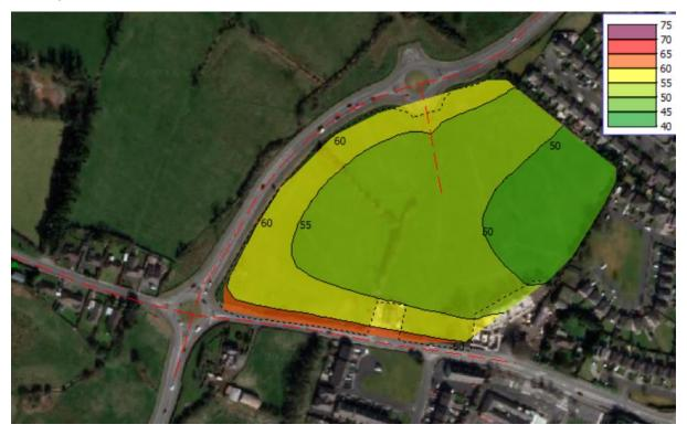
Figure 9.9 Night-time noise contours in dB(A) over existing site – in the absence of the development
